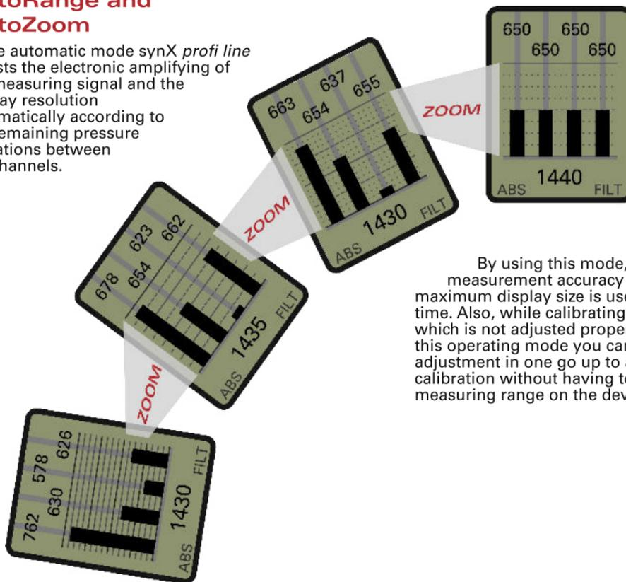
By using this mode, the highest measurement accuracy and the maximum display size is used at any time. Also, while calibrating an engine which is not adjusted properly yet, with this operating mode you can improve the adjustment in one go up to an optimal calibration without having to change the measuring range on the device manually.
